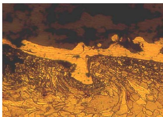
Fig. 2: Image showing deformation and change in grain size in base metal (200X).
