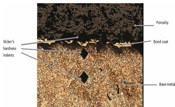
Fig. 1: Microscopic image showing the base metal, bond coat and top coat.
