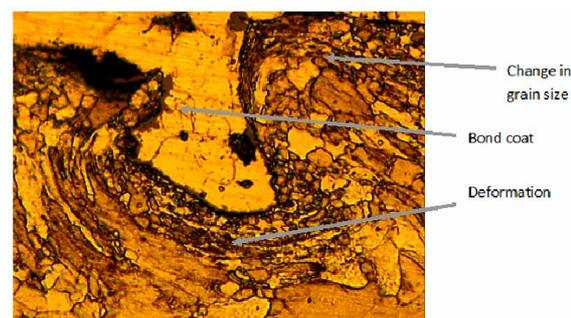
Fig. 3: Detailed view of the deformation caused in the base metal (500X).
