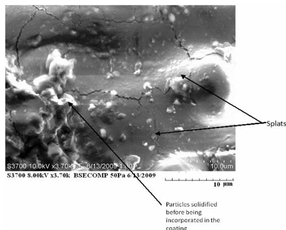
Fig. 5: SEM micrograph of Zirconia Yttria.
