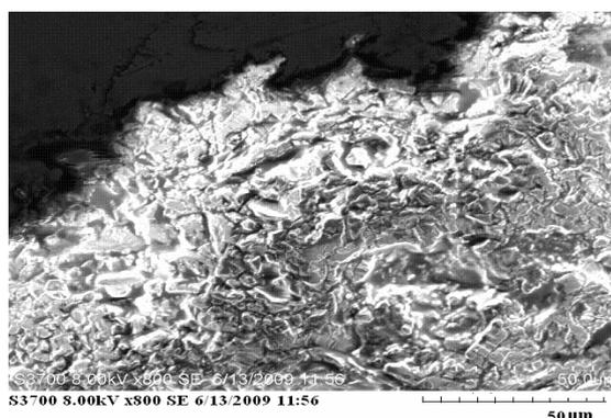
Fig. 4: Top View of NiAl showing lamellar structure.
